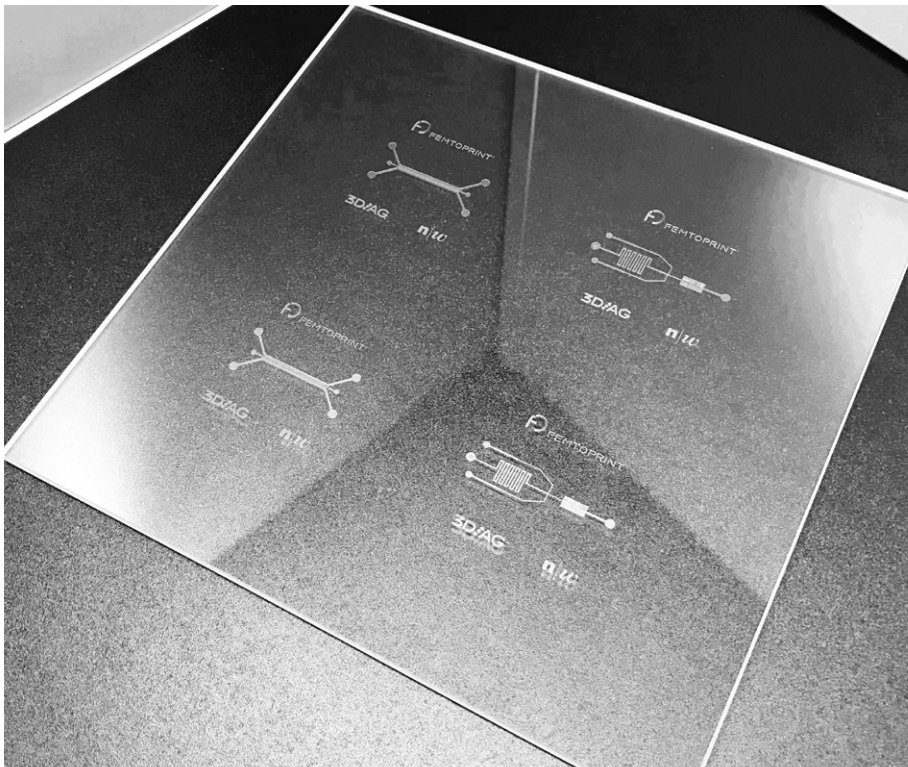
Figure 1. Example of master fabricated on 150 \times 150 \times 3 \text{ mm}^3 fused silica substrate.
